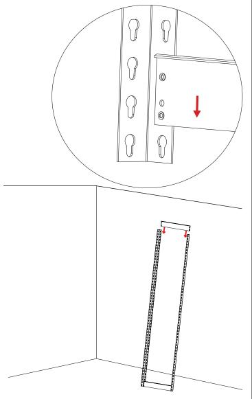
**3.** Assemble another unit end by repeating the directions in step 2. Be sure the shelf support rivets are seated in the bottom of the slots.
