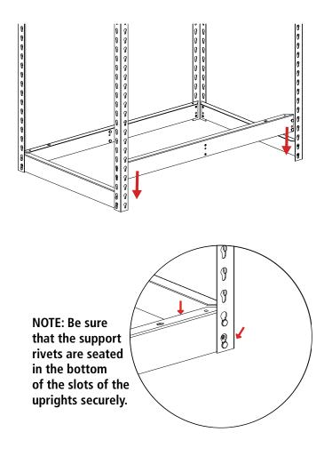
**5.** Finish installing the remaining left-to-right shelf supports and front-to-back shelf supports around the top of the unit as in step 4.
