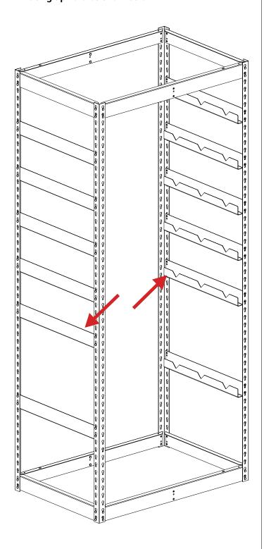
**7.** Rest the reel rod (Ref. No. 5) in the notch of the rod support as shown below. Each rod support level can hold up to three reel rods. Each unit comes with six reel rods.
